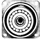
BY SIGHTING THE REAR OF THE GEARING ASSEMBLY, IT CAN BE DETERMINED IF AN ASSEMBLY HAS A SUN DRIVE GEAR OR NOT.
